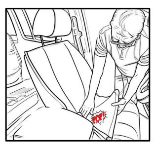
3. While keeping your hand in the seat junction use your other hand to fully unroll the seat bottom portion. Fully extend and use your thumb to push down on the end while your fingers pull up until you hear a "pop". After sitting on your seat cover the front edge of the banding may snap back down. This is normal during use.
